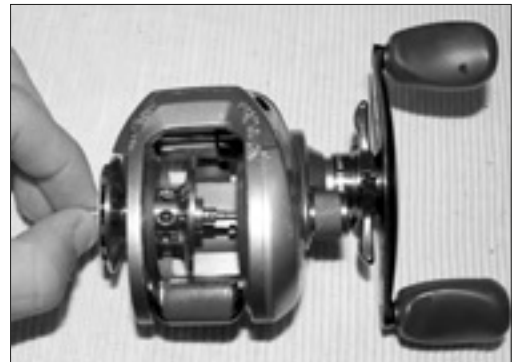
DISASSEMBLY REQUIRED: Breaking down and cleaning a baitcasting reel is a must for saltwater fishermen. The smallest particle of salt can corrode any reel. Photo by Brandon Shuler.
